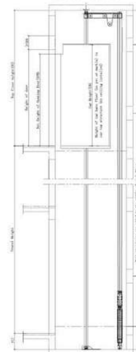
Elevation of Shaft
